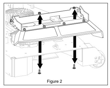
5. 48" and 60" Decks: Remove six tapping screws from deck and retain for operation without mulch kit. See Figures 3 and 4.
