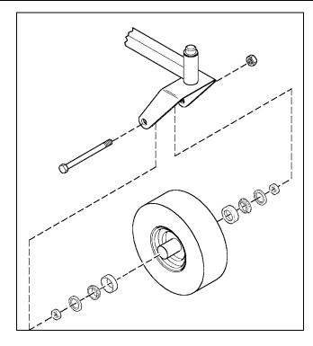
3. Remove locknut (A), cap screw (B), two seal spacers (C) and wheel assembly (D).
