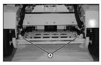
2. Lift machine with a safe lifting device centered under tire support frame (A) on the side where tire is being removed.
