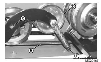
Picture Note: Traction drive belt idler pulley bottom view.
