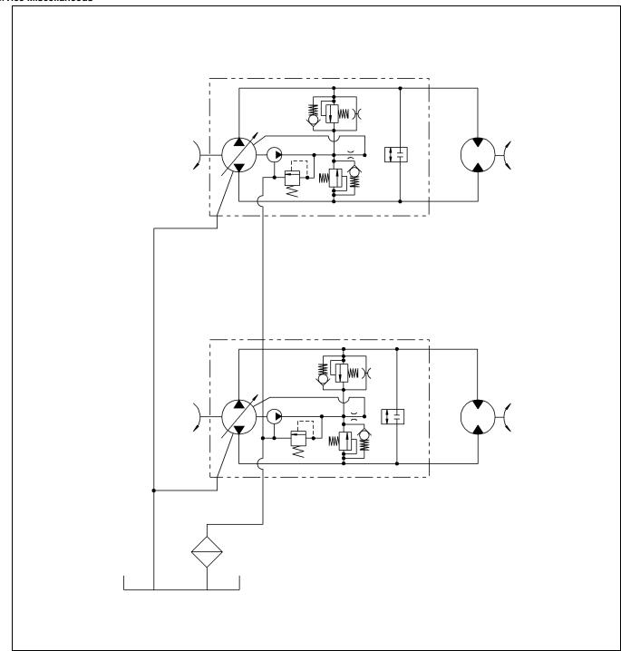
Left Hydrostatic Pump Assembly
