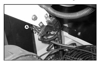
• Open fuse holder (A) and remove socket with fuse.
