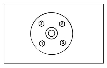
Tighten wheel nuts in numbered sequence shown for safe wheel installation. Tighten alternately until recommended torque value is reached.
