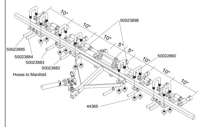
4. In order to have the proper spray pattern please reference the diagram below. The Nozzles need to be approximately ten (10) inches above the ground.
