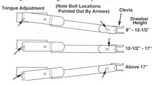
It is important that the FP is operated in a level position. Leveling can be accomplished by adjusting the tractor draw bar height, also by leveling the mower frame by use of the adjustable jack stand.
