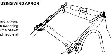
The wind apron is furnished with the unit. This is used to keep the sweepings in the basket on windy days or when sweeping at a fast speed. The wind apron is stretched across the basket and tied on the frame as shown at the top corner and middle at the pivot bracket.
