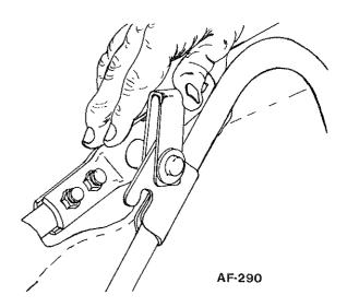
The Wind Apron (AF-291) is furnished with the unit. This is used to keep the sweepings in the basket on windy days or when sweeping at a fast speed. The Wind Apron is stretched across the basket and tied on the frame as shown at the top corner and middle at the pivot bracket.
