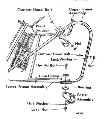
Hold the pivot latch in an up position, then place the pivot rod into the top slot of the pivot bracket. The pivot latch should straddle the bracket. When both sides are resting on the bracket, move the latch forward to lock into position.
