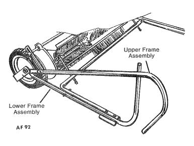
Raise the upper Frame Assembly and match the holes in the lower frame. Fasten with ¼" contour head bolt, lock washer and nut. Do so to both sides. Attach a pivot bracket to each Upper Frame Assembly with a ¼" contour head bolt, lock washer and nut. Be sure the bracket is assembled as shown in Figure 4. The slot for the basket pivot must be above and inside the frame; otherwise the basket will not fit properly.
