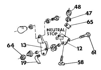
C. Loosen ¼-20 nut (48) holding bracket (12) to handle assembly, until the bracket will slide back and forth in slot.
