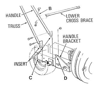
D. Assemble the two handles to top holes of the right and left handle and axle brackets using 5/16-18 x 1-½ bolts and 5/16-18 lock hex nuts. Make sure a steel insert is in the end of each handle as shown when attached at point "D" (above). DO NOT TIGHTEN.
