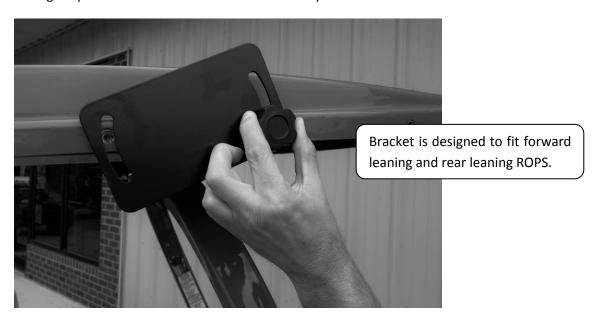
The canopy can be adjusted by user to a forward or aft position for operator's preference. It is important to snug plastic screw knobs securely after adjusting.
