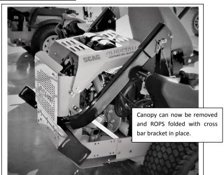
Align top on universal cross bar and install with plastic screw knobs
