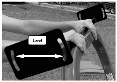
1. Center the universal cross bar on ROPS as pictured. \*\*Notice slot orientation\*\* It is important to position slot to level top properly to your model lawn mower.
