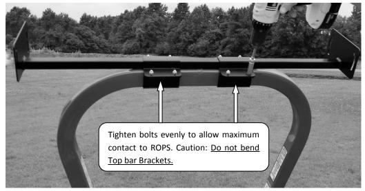
2. Attach using ¼"-20 carriage bolts, ¼" lock nuts, 2 -1"x 1"top bar brackets and the correct ROPS brackets as shown. Make sure the universal cross bar is centered and the ROPS brackets are evenly spaced. It is important to tighten the bolts evenly without bending brackets to allow for maximum contact to all surfaces.
