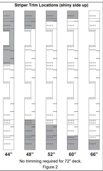
**NOTICE:** Start at one side of the mower deck and install the striper skirt with the glossy rubber side against the mower deck. Depending on the style of the deck, some decks will required drilling holes.
