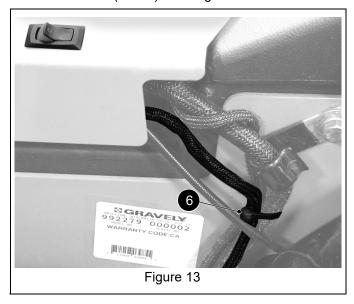
16. Secure headlight harness to frame using four cable ties (item 6). See Figure 14.
