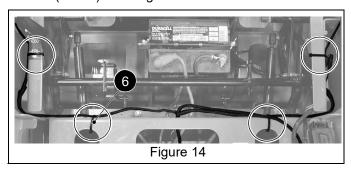
17. Secure left and right headlight harnesses to holes in light mounting arms using two cable ties (item 6). See Figure 15.
