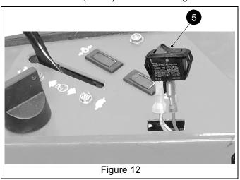
15. Press switch firmly into switch hole until it snaps into position. Secure headlight harness to main harness with cable tie (item 6). See Figure 13.
