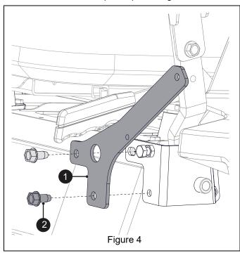
6. Install headlight assembly onto mounting arm using hex bolt, lock washer and hex nut supplied with headlight. Do not fully tighten until headlights are adjusted. See Figure 5.
