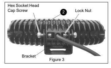
Secure left and right headlights (item 2) to mounting brackets with included hardware. In this application headlights are more effective mounted vertically. Do not fully tighten. See Figure 4.
