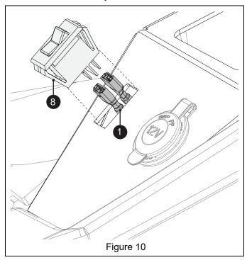
22. Route right headlight harness wire above fans toward right hydraulic reservoir. Secure headlight harness to main harness with two cable ties (item 11). See Figure 11.
