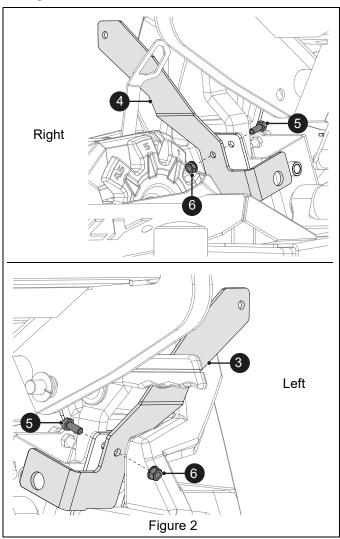
If not pre-installed, secure brackets to headlights (item 2) with included hardware. DO NOT completely tighten hardware until headlights are adjusted. See Figure 3.
