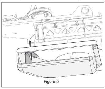
2. Secure baffle with two 3/8" x 3/4" hex bolts (item 6) and two 3/8" nylon top locking flange nuts (item 7). See Figure 6.
