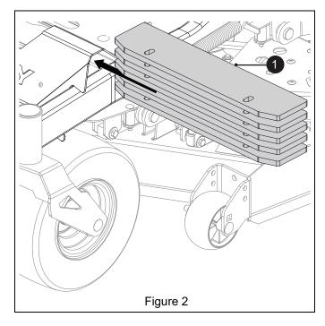
4. Position one counterweight plate under the frame crossmember. Plate is positioned with angled corners facing rearward. Secure weight plates with two 1/2" x 4" hex bolts (item 2), two flat steel washers (item 3) and two 1/2" nylon locking flange nuts (item 4). See Figure 3.
