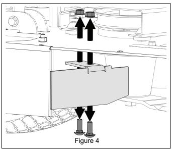
Remove two 5/8" x 1 3/4" hex bolts and Belleville washers retaining blades and remove blades. Note orientation of washers. Retain blades for operation without mulch kit. Retain bolts and washers for kit installation. See Figure 5.
