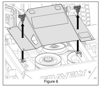
Remove two 5/16" x 1/2" tapping screws from top of deck. Retain screws for operation without mulch kit. See Figure 6.
