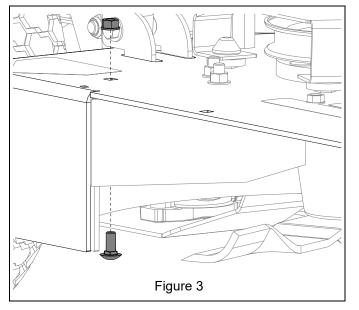
Remove two 3/8" x 1" round head square neck bolts and flanged top lock nuts retaining deflector strip and remove deflector strip. Retain all parts for operation without mulch kit. See Figure 3.
