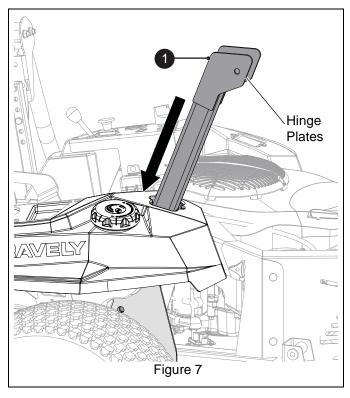
Attach bagger support with one 1/2" x 3 1/4" hex bolt (item 6), one 1/2" x 3" hex bolt (item 5) and two 1/2" top-lock flange nuts (item 7). Fully tighten hardware. See Figure 8.
