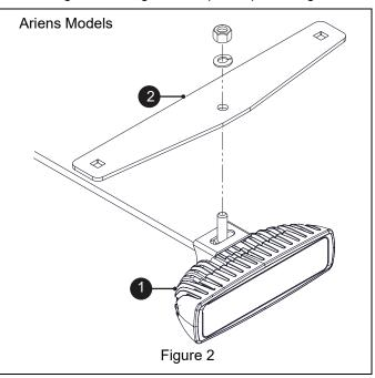
5. Ariens models: Remove and retain two 5/16" locking top flange nuts from bumper mounting brackets. Install headlight assembly (items 1 and 2) on two 5/16 x 3/4" round head square neck bolts and retain with locking top flange nuts just removed. See Figure 3.
