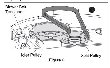
3. Place blower belt tensioner in operating position. **IMPORTANT:** Ensure flat side of V-belt contacts idler pulley and the V-side of V-belt contacts split pulley as shown in Figure 7.
