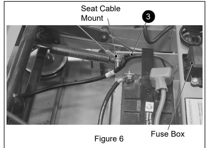
11. Locate purple and black auxiliary wires on unit wire harness under fuse box. Connect red harness wire to purple auxiliary wire. Connect black harness wire to black auxiliary wire. See Figure 7.
