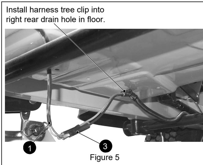
9. Tip seat forward. Route harness between brake lever tube and deck-lift tube and back to fuse box.
