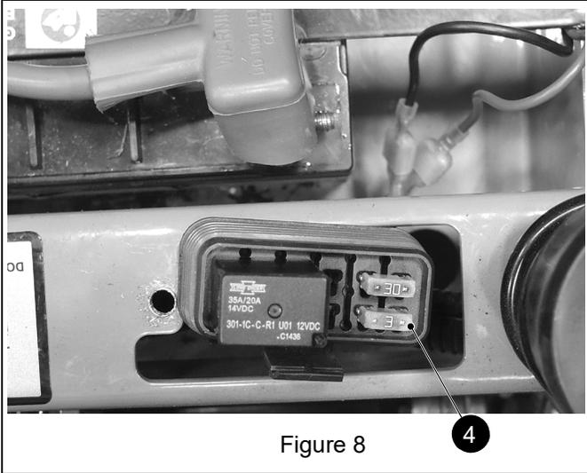
13. Reinstall cover on fusebox and install fusebox in frame.
