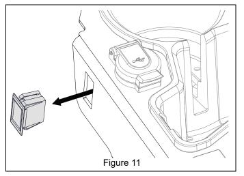
18. Reposition control panel and reconnect USB port and speed selector switch. Route black / white and black wires with flat connectors though switch hole in control panel. Connect spade terminals to rocker switch (item 7). Rocker switch does not have polarity. Wires can be connected to either switch terminal. Secure control panel with fasteners removed earlier. Do not fully install switch yet. See Figure 12.
