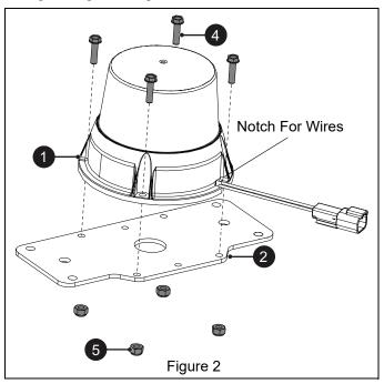
Secure light assembly to ROPS using two 5/16" x 3/4" hex washer head tapping screws (item 3). See Figure 3.
