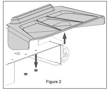
5. Remove two 5/16 x 3/4" round head square neck bolts and two 5/16" locking flange nuts retaining discharge baffle and remove baffle. Retain baffle and hardware for operation without mulch kit. See Figure 3.
