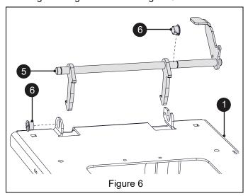
4. Install seat latch into seat plate assembly. Ensure that bushing flange on latch is positioned on the outside of the seat bracket. See Figure 7.
