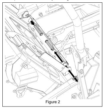
4. Remove and retain two 5/16" bolts retaining coupling nuts, compression springs and spacers. Dispose of coupling nuts, compression springs and spacers. See Figure 3.
