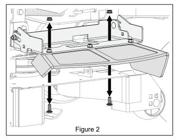
5. Remove six tapping screws from deck and retain for operation without mulch kit. See Figure 3, 4, or 5.
