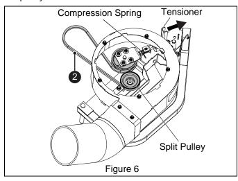
**IMPORTANT:** Ensure flat side of V-belt contacts idler pulley and the V-side of V-belt contacts split pulley as shown in Figure 7.
