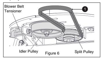
3. Place blower belt tensioner in operating position. **IMPORTANT:** Ensure flat side of V-belt contacts idler pulley and the V-side of V-belt contacts split pulley as shown in Figure 7.
