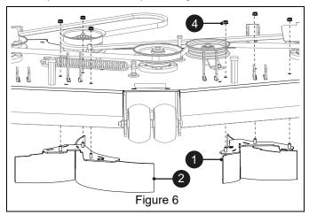
Position discharge baffle (item 3) in mower deck and retain with two 5/16" center lock flange nuts (item 4). Torque nuts to 9.1 N•m – 10.2 N•m (80 lb-in – 90 lb-in). See Figure 7.
