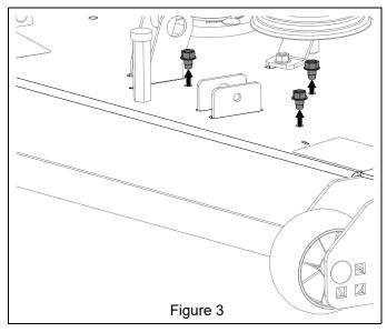
6. Remove and retain three 3/8" x 1/2" tapping screws from right side of deck. Reinstall tapping screws when operating mower without mulch kit. See Figure 4.
