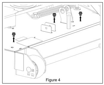
Remove and retain three 5/8" x 1 3/4" hex bolts and washers retaining mower blades and remove mower blades. Note bevel washer orientation for reinstallation. Retain hardware for reinstallation and blades for operation without mulch kit. See Figure 5.
