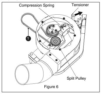
3. Place blower belt tensioner in operating position. **IMPORTANT:** Ensure flat side of V-belt contacts idler pulley and the V-side of V-belt contacts split pulley as shown in Figure 7.
