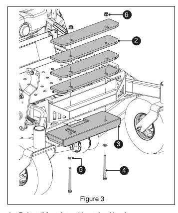
4. Reinstall footplate with retained hardware.
