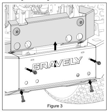
Align hitch plate (item 1) with holes in bumper.
