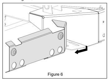
Align hitch plate (item 1) with holes in bumper.
