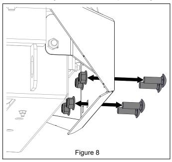
5. Align hitch plate (item 1) with holes in bumper and secure with four 1/2" x 1 1/2" hex bolts (item 3) and four 1/2" nylon locking flange nuts (item 4). See Figure 9.
