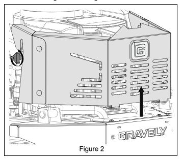
4. Remove and retain hex bolts retaining heat shield to bumper and remove heat shield or move out of the working area. See Figure 3.
