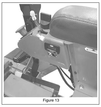
12. Connect switch (item 3) to wires. See Figure 14. **NOTICE:** Headlight switch does not have polarity. Purple and blue wires may be connected to either switch port.
