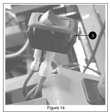
13. Press switch firmly into hole until it snaps into position. Ensure that red side of rocker in switch faces to the rear. See Figure 15.
