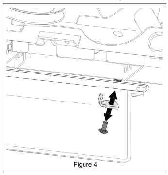
7. Install bagger discharge bracket (item 9) in front of blower housing outlet. Secure with one 5/16" x 3/4" round head square neck bolt (item 10) and one 5/16" center locking flange nut (item 11). See Figure 5.
