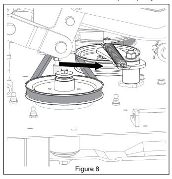
4. Remove 3/8" hex bolt and sheave retainer from top of spindle. Remove pulley. Discard pulley and hex bolt. DO NOT discard sheave retainer. See Figure 9.
