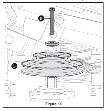
2. Reinstall mower drive belt and reconnect idler arm spring.
