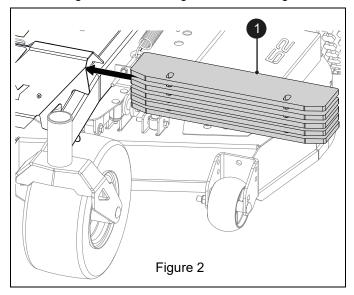
5. Position one counterweight plate (item 1) under the frame crossmember. Plate is positioned with angled corners facing rearward. Secure weight plates with two 1/2" x 4" hex bolts (item 2), two flat steel washers (item 3) and two 1/2" nylon locking flange nuts (item 4). See Figure 3.
