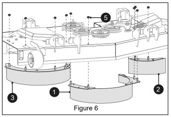
Install three mulch blades (item 4) with Belleville washers and hex nuts removed earlier. Ensure that cupped faces of washers face blades. Torque blade nuts to 136 N•m – 163 N•m (100 lb-ft – 120 lb-ft). See Figure 7.
