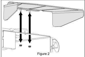
Remove two 5/16" x 3/4" round head square neck bolts and flanged top lock nuts retaining deflector strip and remove deflector strip. Retain all parts for operation without mulch kit. See Figure 3.
