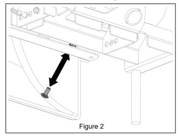
Install bagger discharge bracket (item 2) in front of blower housing outlet. Secure with one 5/16" x 3/4" round head square neck bolt (item 3) and one 5/16" center locking flange nut (item 4). See Figure 3.
