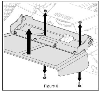
8. Remove belt cover from mower deck. Retain for operation without bagger. See Figure 7.
