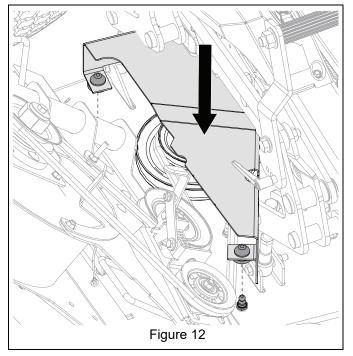
16. Install blower belt cover onto bracket and secure with one 1 1/2" washer and one knob from bagger kit. See Figure 13.
