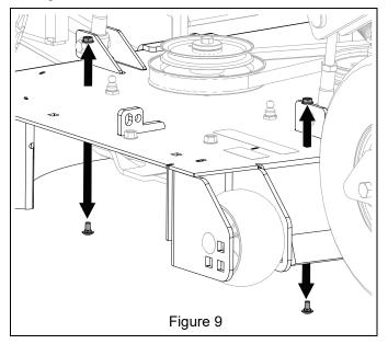
11. Attach two threaded ball studs (item 7) to deck using bolts just removed. See Figure 10.
