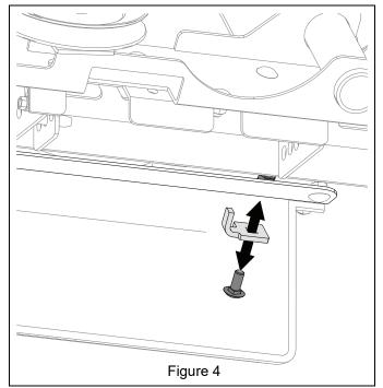
Install bagger discharge bracket (item 9) in front of blower housing outlet. Secure with one 5/16" x 3/4" round head square neck bolt (item 10) and one 5/16" center locking flange nut (item 11). See Figure 5.
