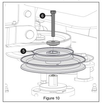
2. Reinstall mower drive belt and reconnect idler spring.
