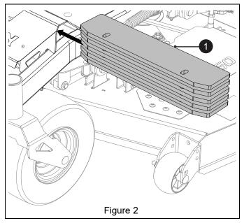
Position one counterweight plate under the frame crossmember. Plate is positioned with angled corners facing rearward. Secure weight plates with two 1/2" x 4" hex bolts (item 2), two flat steel washers (item 3) and two 1/2" nylon locking flange nuts (item 4). See Figure 3.
