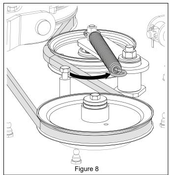
Remove 3/8" hex bolt and sheave retainer from top of spindle. Remove pulley. Discard pulley and hex bolt. DO NOT discard sheave retainer. See Figure 9.
