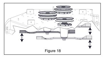
If the front measurement is not 3.2 mm (1/8") lower than the rear measurements, adjust the blade pitch. See *Adjust Blade Pitch* on page 7.
