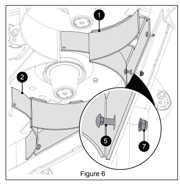
Secure top of each baffle to deck with one 5/16" x 1" hex bolt (item 6) and one 5/16" nyloc flange nut (item 7). See Figure 7.
