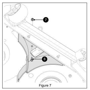
3. Secure discharge baffle (item 3) to deck with two 5/16" nyloc flange nuts (item 7). See Figure 8.
