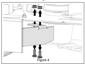
7. Remove two 5/8" x 1 3/4" hex bolts and Belleville washers retaining blades and remove blades. Note orientation of washers. Retain blades for operation without mulch kit. Retain bolts and washers for kit installation. See Figure 5.
