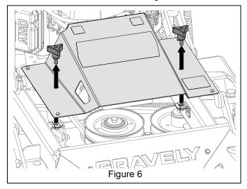
9. Remove two 5/16" x 1/2" tapping screws from top of deck. Retain screws for operation without mulch kit. See Figure 6.
