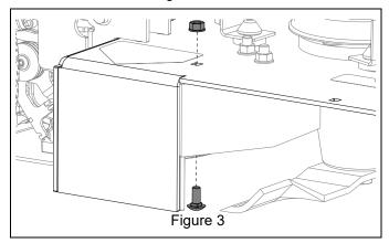
6. Remove two 3/8" x 1" round head square neck bolts and flanged top lock nuts retaining deflector strip and remove deflector strip. Retain all parts for operation without mulch kit. See Figure 3.
